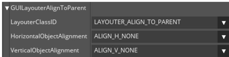
This Layouter aligns the attached object relative to its parent object.
