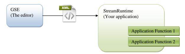
There is the GSE on one side, in which you graphically design your user-interface by placing controls, assigning bitmaps, changing texts etc.
