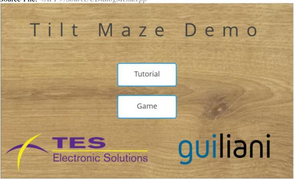
This dialog only contains two buttons, which are used to change to the appropriate screen. As explained in 5.3 to change the screen in the tilt maze demo, only a single *CallAPI*-Command needs to be called. This is done in the GSE, so the *CDialogMenu* class is quite barebones.
